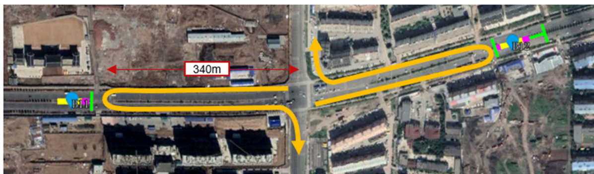
Figure 32: Proposed change from 3 to 2 phases by using u-turns already in the project design.
